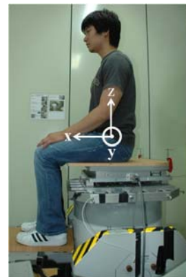
Fig. 2 Photographic representation of vibration shaker and subject sitting on the rigid seat
